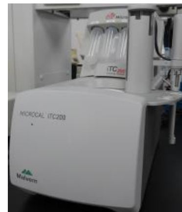
Thermodynamics assay with ITC
